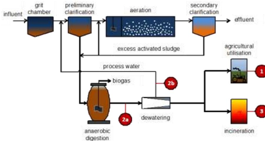
**Legend:** 1 = direct sludge (biosolids) application in agriculture; 2a = P recovery from aqueous sludge phase prior to dewatering; 2b = P recovery from sludge liquor after dewatering; 3 = P recovery from mono-incineration ash.
