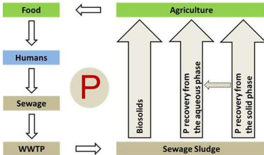
**Figure 3:** The three principal routes for P recovery and recycling from the wastewater stream as a nutrient. Wastewater REUSE for irrigation is not included. (Kabbe, 2013).
