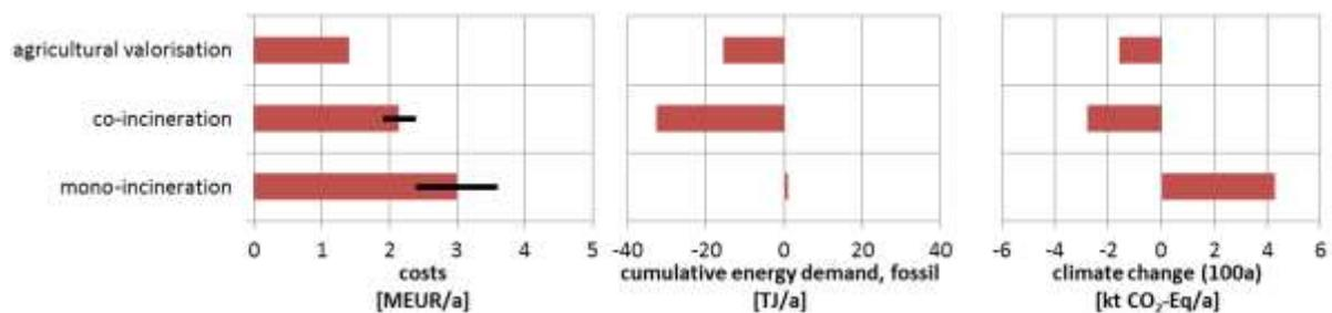
**Figure 7: costs, fossil cumulative energy demand and climate change (100a) for different sludge disposal routes for a 1 million p.e. waste water treatment plant (P-REX reference system)**
