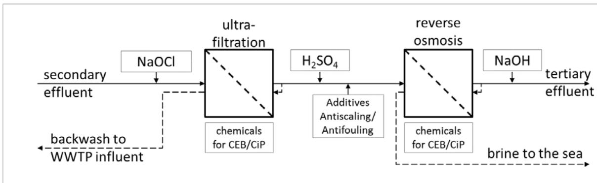
Figure 9 Basic flow sheet of Ultrafiltration (UF) and reverse osmosis (RO)
