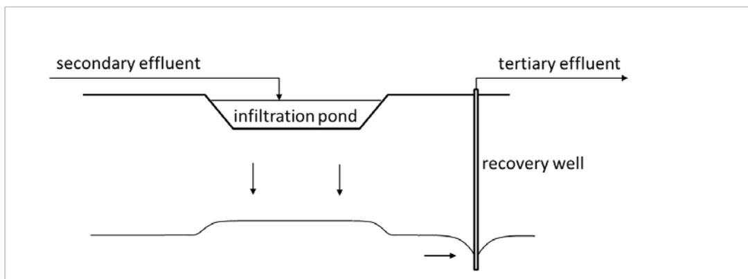
Figure 6 Basic flow sheet for SAT treatment
