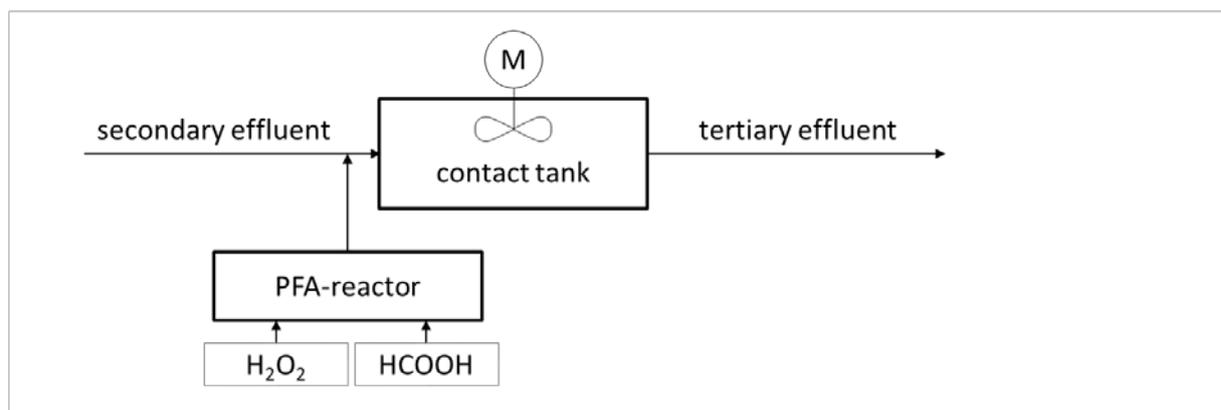
Figure 2 Basic flow sheet for PFA disinfection
