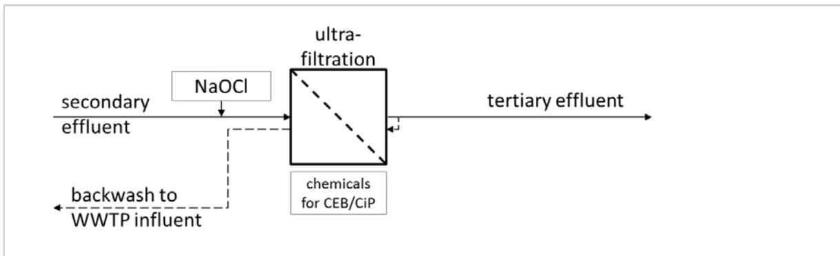
Figure 8 Basic flow sheet for ultrafiltration (UF)
