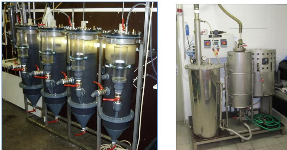
**Figure 2: Lab-scale digesters (40L) for pilot trials of co-digestion and equipment for thermal hydrolysis**
