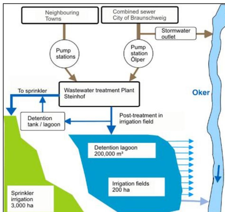
Figure 1: Simplified representation of the Braunschweig sanitation scheme.
