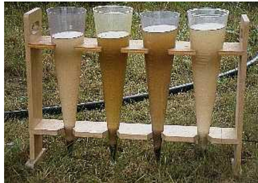
Figure 5: Imhoff cones [www.geologie-franken.de]
